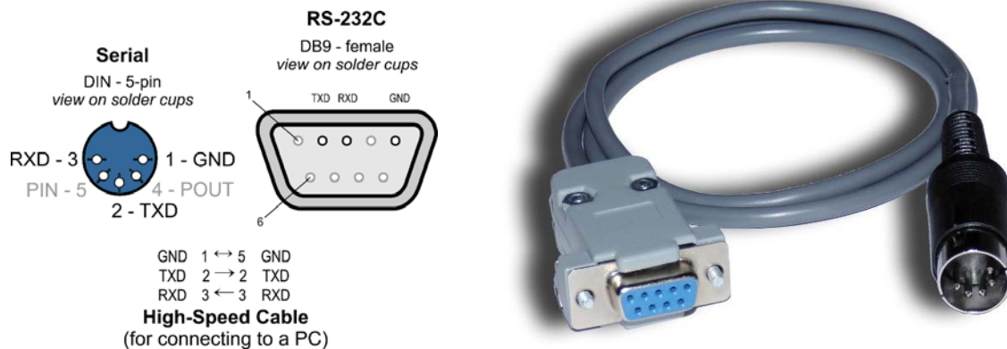
Figure 18: Cable to connect to HX-20 to a PC running the MH-20 screen and disk emulator. Only 3 wires are needed.
