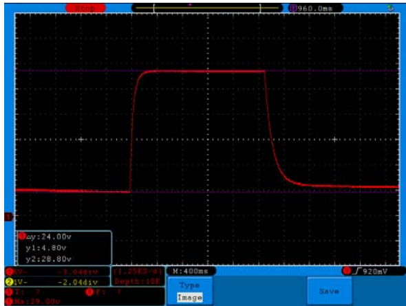
Figure 9: Configuration 1: Zener Diode ZD5 clipped, ROMs removed.
