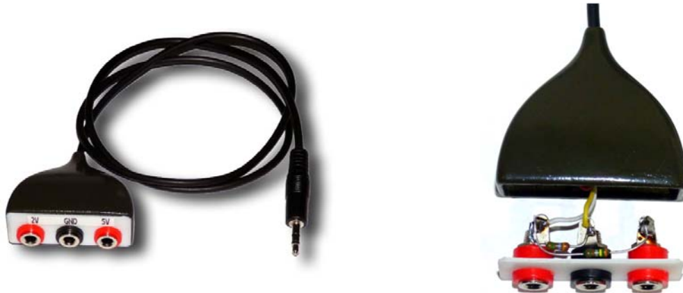
Figure 15: Cable and plug box to connect 2 V or 5 V to the ADC input. The two resistors (e.g. 3.47 k \Omega and 2.3 k \Omega ) must have a ratio of 1.5 to reduce 5V to 2V.
