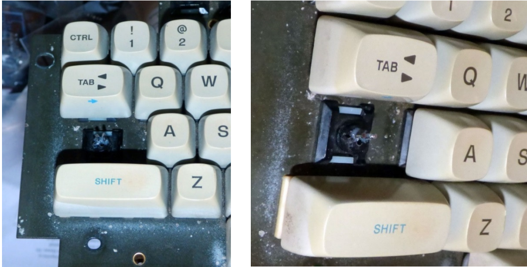
Figure 8: Keyboard with missing key and steel pins already glued into the plunger.
