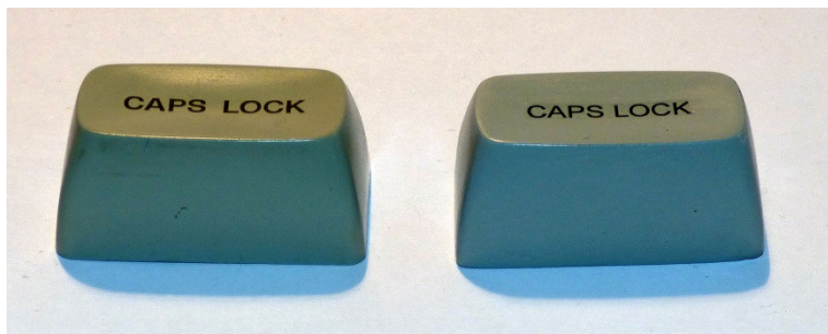
Figure 12: Key caps: left original, right: reproduction, painted and with decal applied, but not yet coated with clear protective layer.
