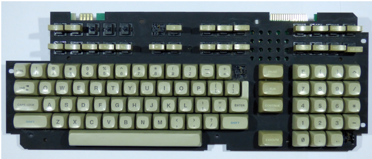
Figure 20: Keyboard with broken switches taken off. Note that one of the function keys in the upper right is also almost broken and leans forward.
