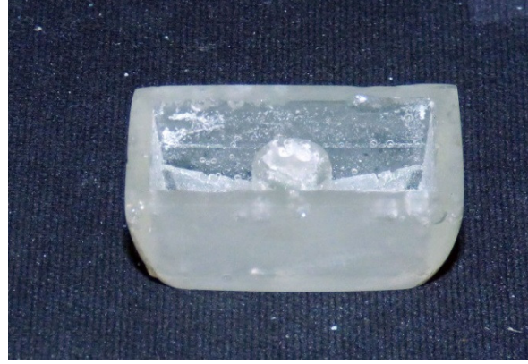
Figure 10: The key cap as cast in clear epoxy resin with the casting spruce removed and slightly wet sanded.
