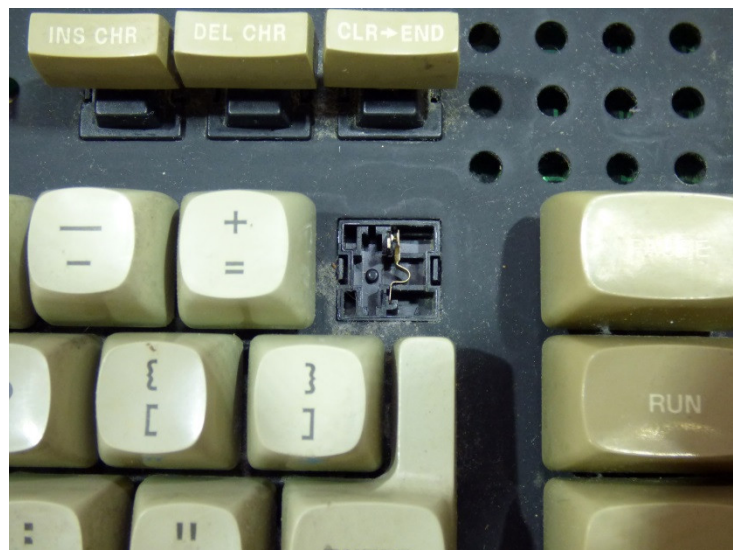
Figure 21: Enlarged view of a broken switch. The upper part of the switch case seems to be welded ultrasonically to the lower part and this connection breaks.
