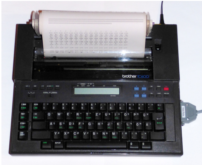
Figure 2 A Brother TC-600 with German keyboard, serial cable and power supply connected. The paper holder for Fax paper rolls has been built by myself. A similar holder had been available as an accessory (order #6600). Furthermore, my machine is missing the keyboard and the serial port covers.
