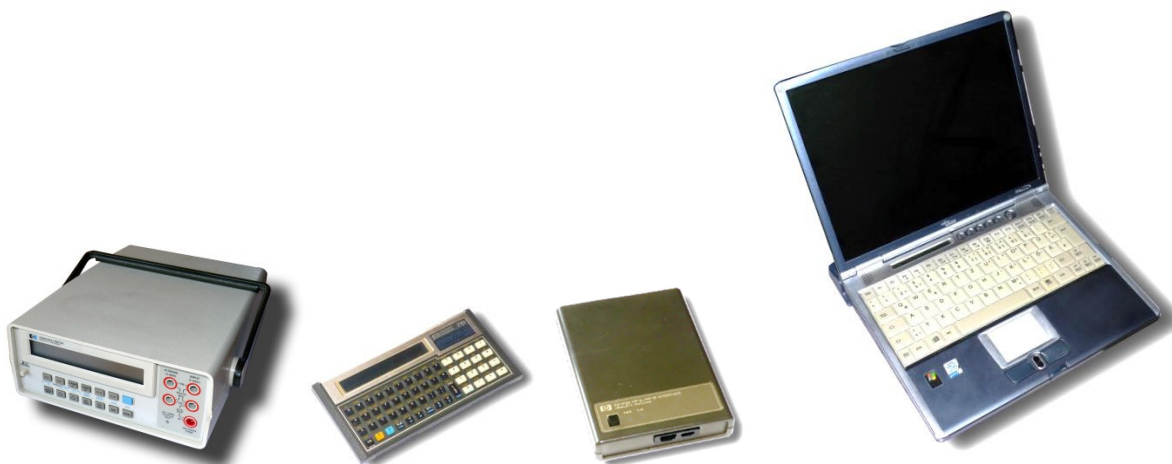
Figure 3: Processing chain: HP 3468A, HP 71B, HP-IL–HP-IB converter and Laptop.
