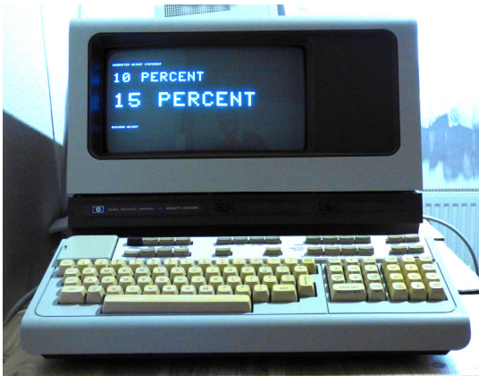
Figure 6: Text Size. The HP 2648A uses a scalable, pixel based font.
