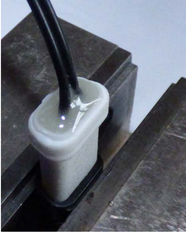
Figure 11: Housing with pins and cable completely filled with epoxy. Do not overfill as the end cap volume is limited. The upright position allows filling the recess to properly grab the insulation of the cable.
