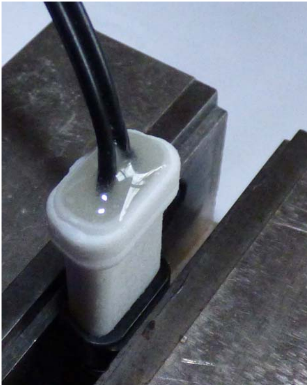
Figure 12: Housing with pins and cable completely filled with epoxy. Do not overfill as the end cap volume is limited. The upright position allows filling the recess to properly grab the insulation of the cable.
