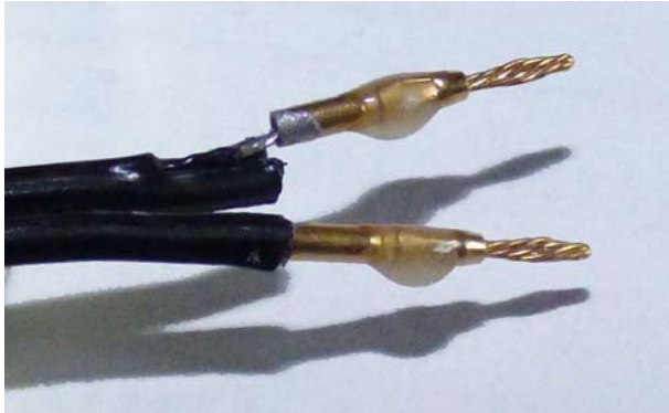
Figure 8: Male connector pins with fresh Epoxy applied, seconds before being inserted into the housing. Be careful to avoid the application of Epoxy to the part of the connector pins forward of the conical section.
