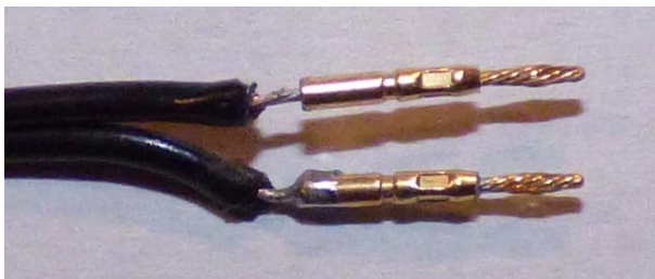
Figure 8: The wires soldered to male pins. The lower pin receives too much solder which had to be removed to fit the assembly into the housing. Note: if you have a suitable crimp tool, use this instead of soldering.
