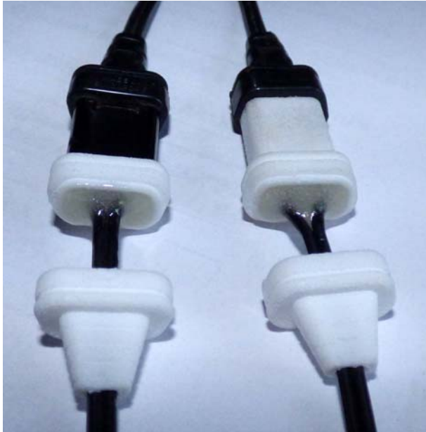
Figure 12: Both ends are ready to be mated to their end caps. I keep the original HP-IL cable attached for aligning the pins as long as possible – even the 5-minute Epoxy needs about 24 hours to cure completely.
