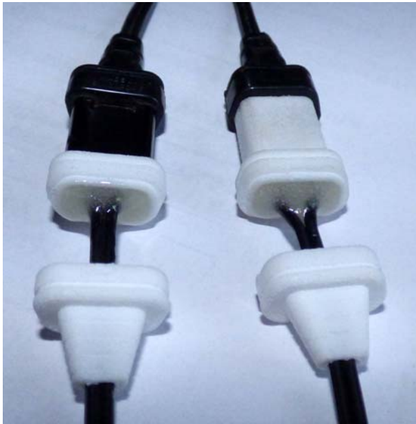
Figure 13: Both ends are ready to be mated to their end caps. I keep the original HP-IL cable attached for aligning the pins as long as possible – even the 5-minute Epoxy needs about 24 hours to cure completely.
