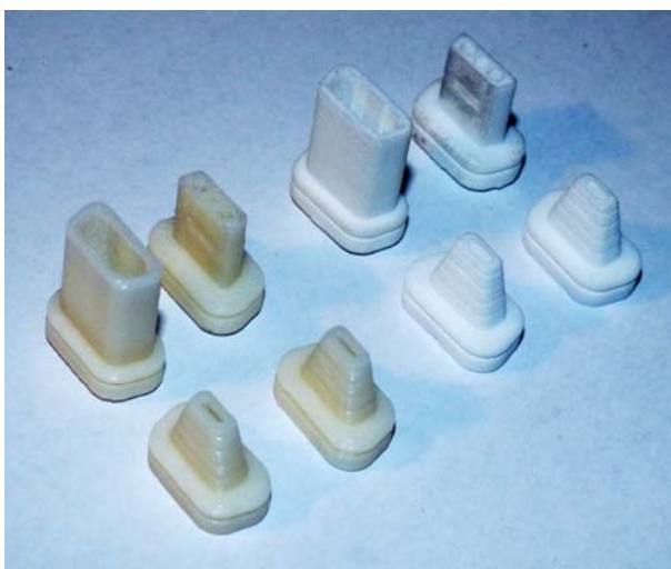
Figure 5: 3D-printed plastic parts. The cream colored parts on the left are made from extruded ABS while the white parts on the right are sintered polyamide.
