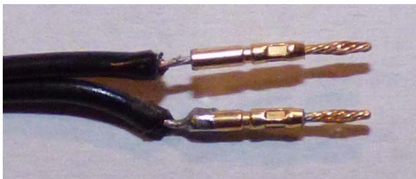
Figure 7: The wires soldered to male pins. The lower pin receives too much solder which had to be removed to fit the assembly into the housing. Note: if you have a suitable crimp tools, use this instead of soldering.
