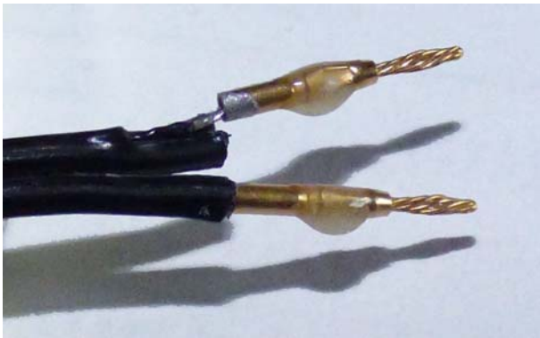
Figure 9: Male connector pins with fresh Epoxy applied, seconds before being inserted into the housing. Be careful to avoid the application of Epoxy to the part of the connector pins forward of the conical section.
