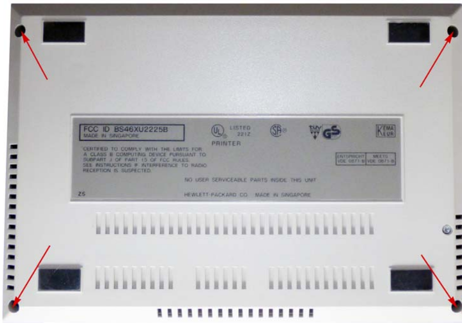
Figure 10 Opening the case requires nothing more than removal of these four screws. The additional screw holds the chassis in place and will be removed later.
