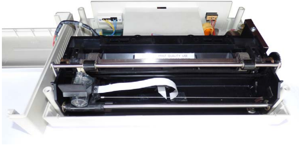
Figure 18 The Flexprint cable can be pre-bent to keep it in the desired shape. Note the plastic clip clamping its end to the chassis bottom. You can see a loop of the Flexprint adapter ribbon cable peeking out over the front edge of the battery box – it could have been shorter. On the other hand this loop allows placing the ZIF connector into the space between chassis and battery box without interference or risk of short circuits.
