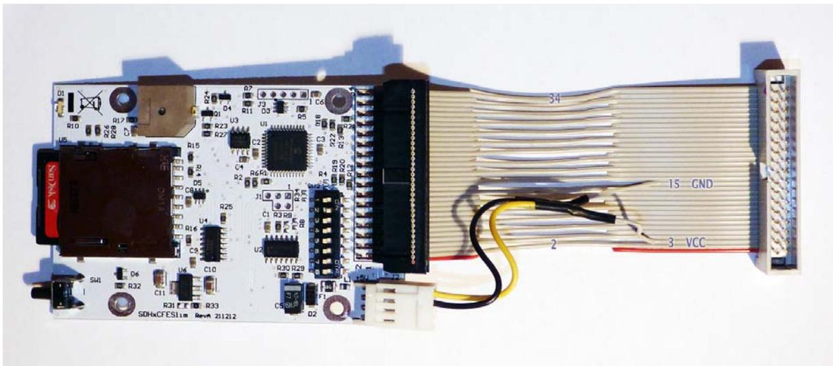
**Figure 2:** Adapter cable with power supply lines. All odd lines except 3 and 15 are cut. All lines with even numbers are connected to the upper row on the HxC connector. The plug on the original cable in the HP 9153 system is plugged into the connector at the right hand side.
