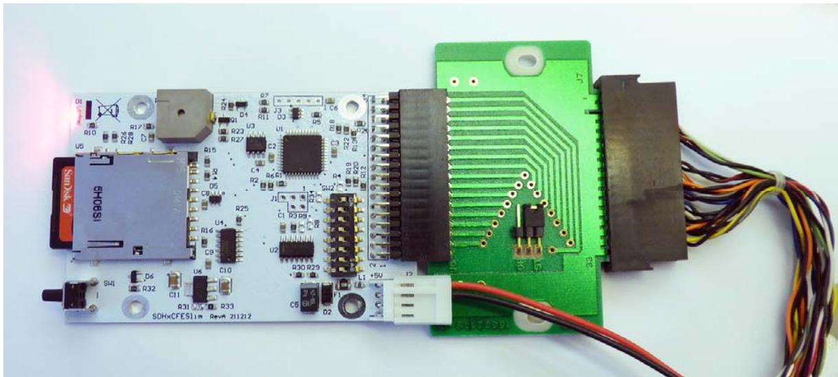
**Figure 8:** A simple adapter was used to connect the HxC Emulator to the edge connector provided by the HP 86A computer. These adapters were supplied in the 1980s with TEAC 3.5" floppy disk drives. The power supply is connected to the separate 5V/12V connector.
