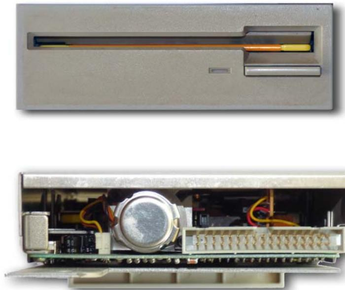
**Figure 1: Front and rear view of SONY MFD-52-W10 flexible disk drive. Note that there is no separate power connector.**
