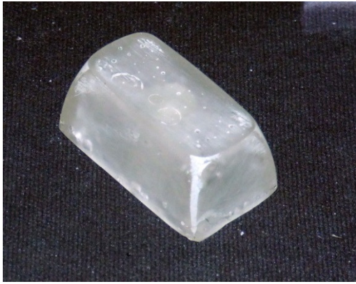
Figure 10: The key cap as cast in clear epoxy resin with the casting spruce removed and slightly wet sanded.
