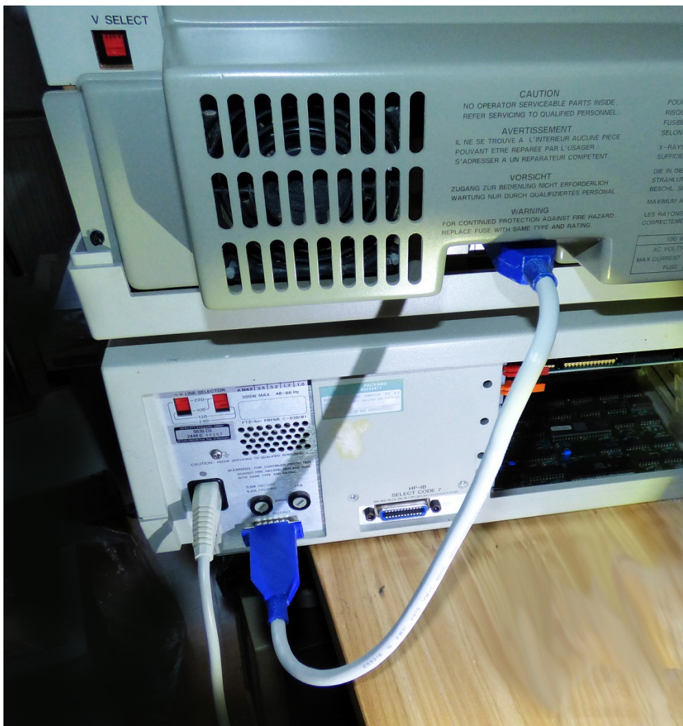
Figure 26: The new cable installed. The upper connector is secured to the monitor with two screws. The lower connector (which should have a sliding lock), is just held in place by friction.
