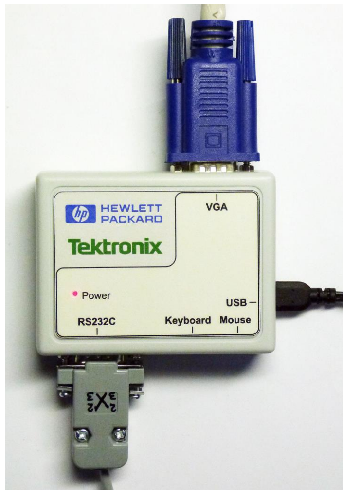
Figure 5 The completed terminal for Tektronix and HP terminal emulation.
