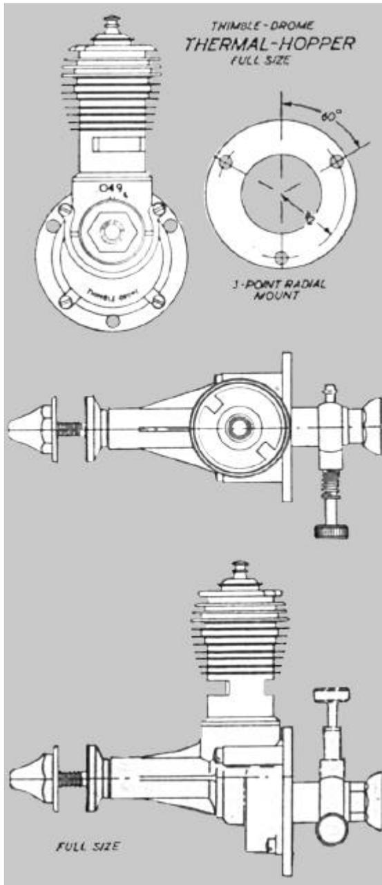
**T**HE Thermal-Hopper came in for test with quite a reputation behind it. In the first place it is a novelty from the design point of view in employing crankcase induction controlled by a reed valve. In the second place quite fantastic r.p.m. figures are claimed by the manufacturers and, thirdly, it is claimed as the fastest starting engine in its class. Like the majority of American production engines it has glow plug ignition.
