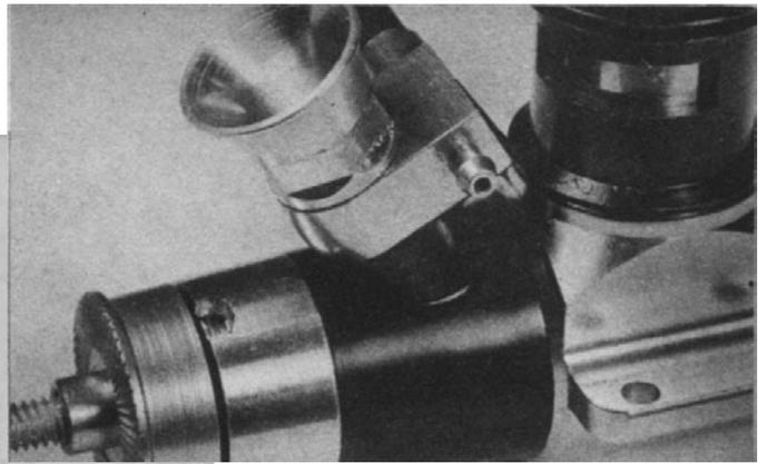
Front rotary induction with a difference is the key to the new high performance in .15 engines.
