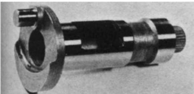
Massive 7/16" journal, equals big valve port, better volumetric efficiency, power.
