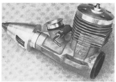
align the two parts. Four long screwspass through the jacket from the cylinder head to tie the complete cylinder assembly to the crankcase. The piston and conrod assembly are fairly conventional. The lightweight lapped cast-iron flat-crowned piston has a thin skirt and small bosses and is coupled to a forged aluminium connecting-rod by a hollow gudgeon-pin retained by wire circlips.
