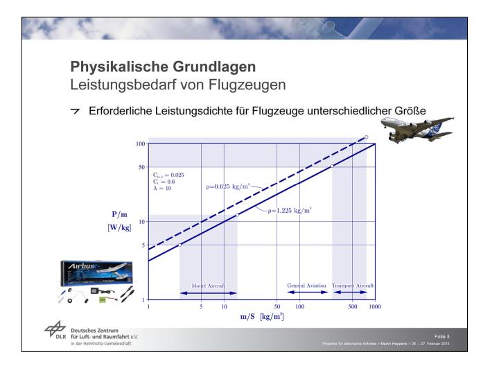
Not everything is easily scalable. The graph shows the required power per mass over wing loading. Small and slow aircraft have much lower wing loadings than heavy and fast aircraft. This is a result of the so called square-cube scaling law.
